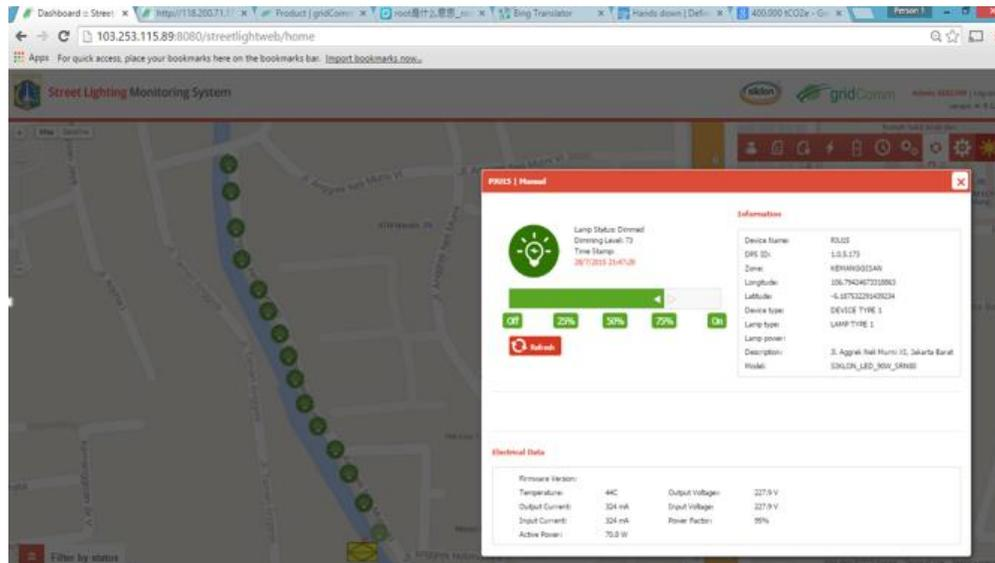
Figure 4 – Manual Control to Turn ON/OFF/Dim Street Light
