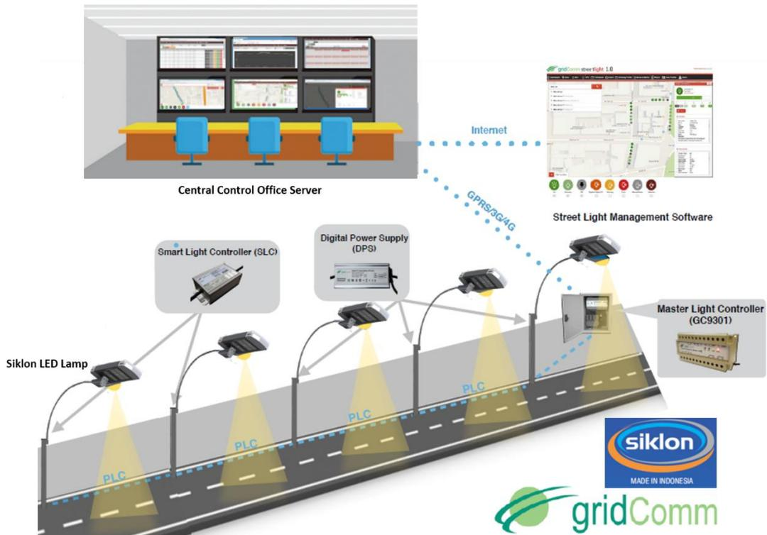
Figure 2 – gridComm-Siklon Smart Street Light System
